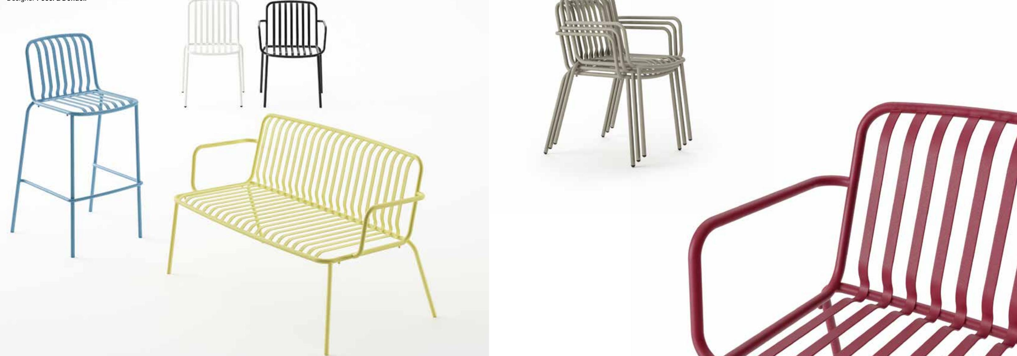
**Stilo** is a complete collection consisting of 5 models, which are meant for outdoor as well as indoor environments, they are completely made of steel tube and rounded steel plate; the production processes are managed by machines at CNC control so as to guarantee continuous quality. The single metallic parts are joined with the TIG welding technology, which does not produce any residual or scrap and the elements are perfectly merged together.
